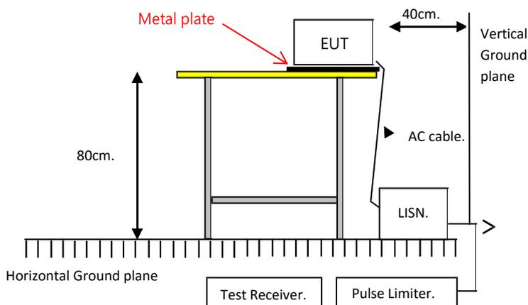
Figure 1 : System Deployment of EMI Test
